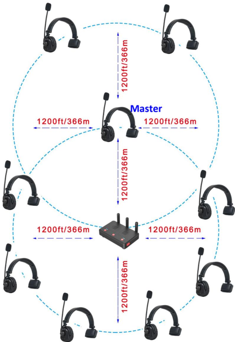
From the observation of above diagram, each remote headset can be replaced with the hub to increase the number of the remote headsets and extend the working distance.
